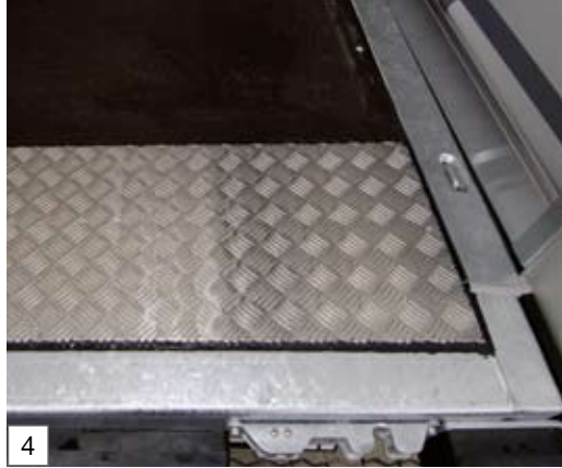
Wear plate at the end of the floor minimises floor damage from abrasive loads
