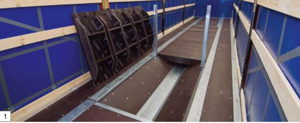
A special completely galvanised well and steel stanchions provide a secure holding for steel coils. With the well covering, the well can be closed when being used for transporting normal products
