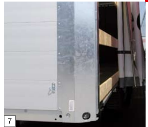
7 Galvanised steel corner supports for increased body strength
