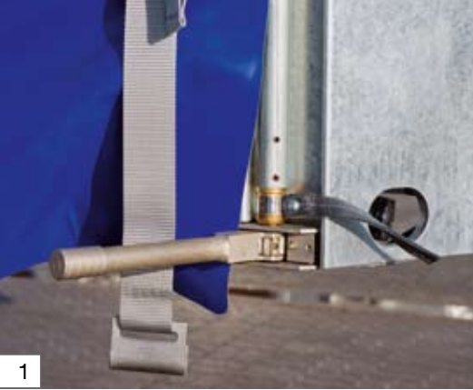
1 Front release device for quick opening and closing of the side tarpaulins
