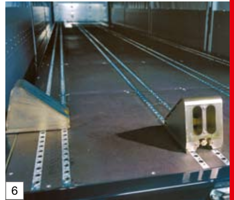
Four pairs of perforated rails fitted in the floor over the whole vehicle length with load securing wedges
