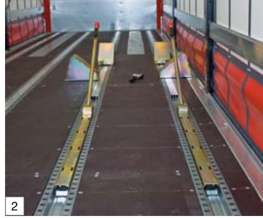
Continuous steel rails for the Joloda rollers with locking mesh for safety wedges
