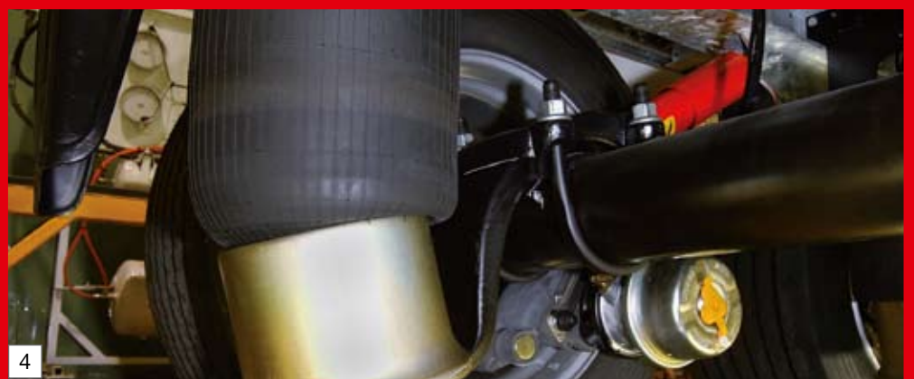
Variable: the MRH air suspension with two driving heights for the different coupling heights
