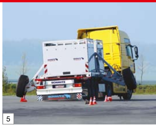
Safety in every position – the integrated RSP electronic stability program ensures safe braking in a curve during critical situations
