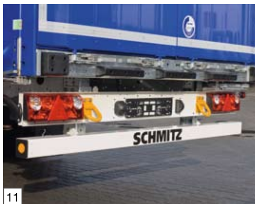
Retrofittable, bolted ferry rings for safe sea transport
