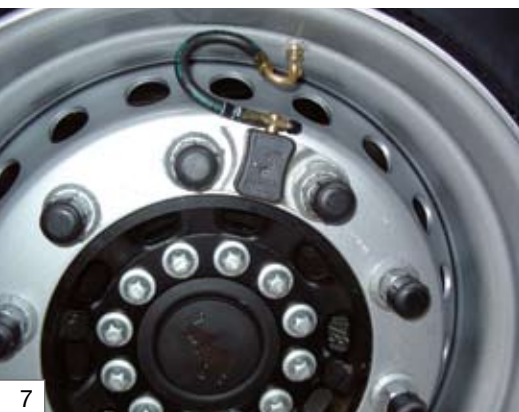
7 Tyre pressure control system, increases the mileage and reduces tyre damage
