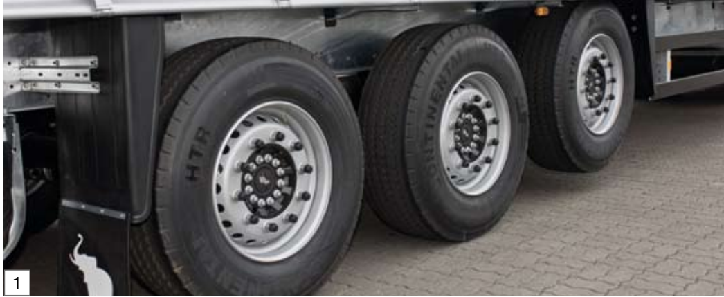
1 Front axle lift with automatic lifting and lowering
