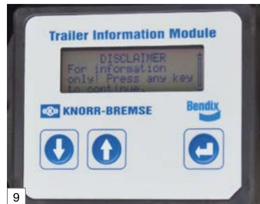
8 Trailer information system for displaying vehicle data, such as axle load, brake pad wear and mileage
