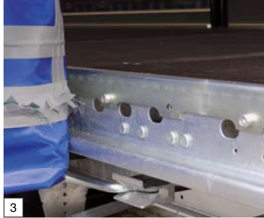
Through load-securing holes in the outer frame
