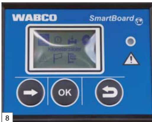
8 Trailer information system for displaying vehicle data, such as axle load, brake pad wear and mileage
