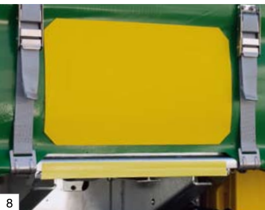
Bolted gripping strips for the combined traffic, flatbed fittings can be retrofitted
