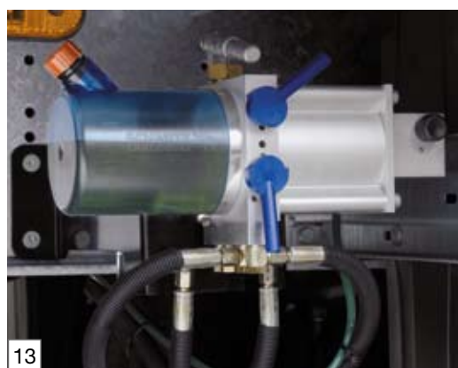
13 Hydro-pneumatic pump for comfortably raising the roof to the left, right or on both sides
