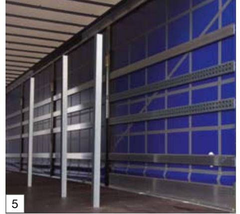
Eight pairs of additional stanchions can be inserted in the central/outer stanchion pockets
