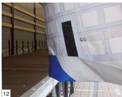
12 Velcro fastener in the tarpaulin for adapting to the different body heights
