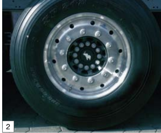
Aluminium rims reduce the empty weight and increase the value of your vehicle
