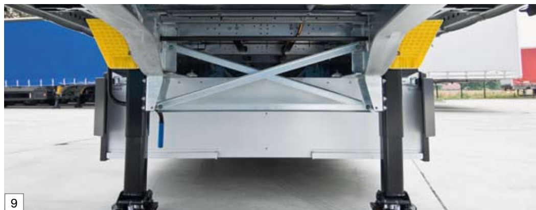
Hot galvanised chassis The galvanising of all components already ensures for a high value stability before bolting
