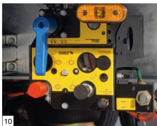
Compressed air-operating unit with AUTO-RESET stability program reduces bellow damage
