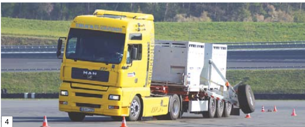
Safety in every position The integrated electronic stability program RSP ensures safe braking in a curve during critical situations.
