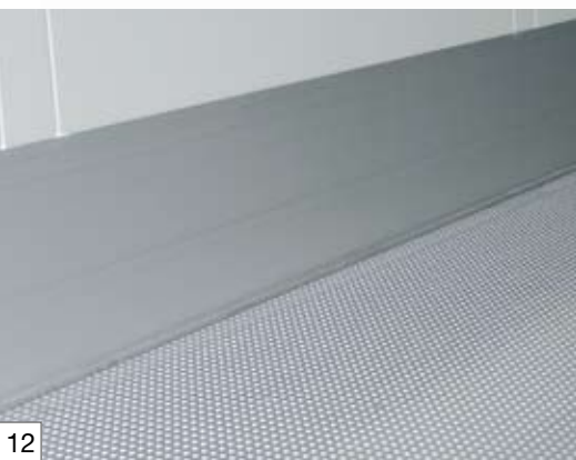
Aluminium grooved plate with floor pan including frame scuff rails
