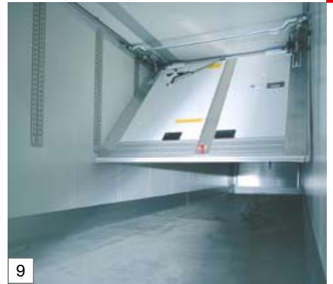
Longitudinally displaceable, insulated transverse partition panel
