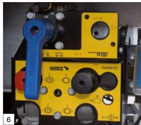
Running gear operating unit with AUTO-RESET function
