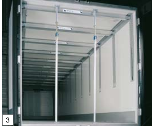
Telescopic cargo bars, both sides fitted with rubber feet
