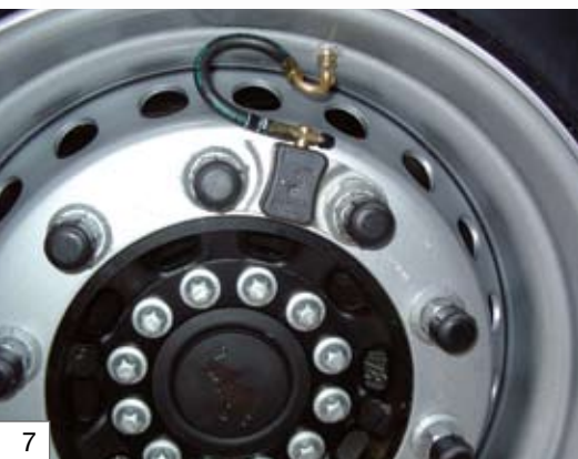
Tyre pressure control system, increases the mileage and reduces tyre damage
