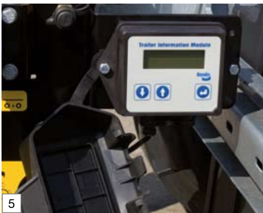
TIS (Trailer Information System) optional with hub-odometer and axle load display, optional with brake pad wear indicator
