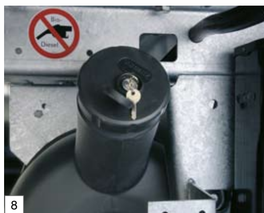
Plastic diesel tank with lockable tank cap
