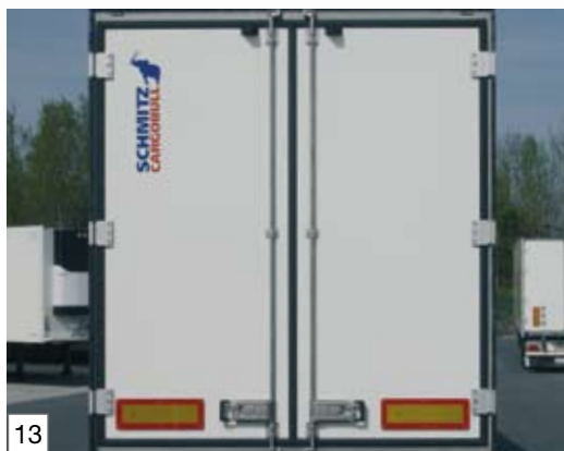
Rear doors made from FERROPLAST®
