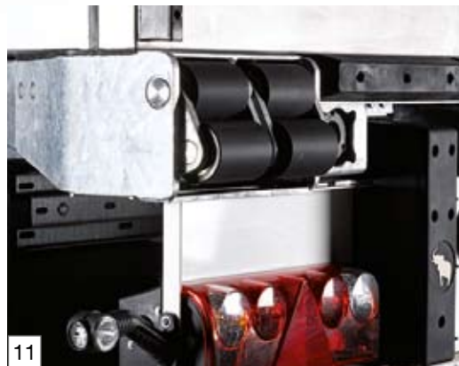
Compression roller rubber bumper for the effective shock absorption when making contact with the ramp
