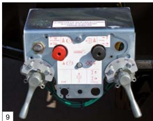
Control unit for parking brake and pneumatic suspension with 2 lifting & lowering valves and container locking
