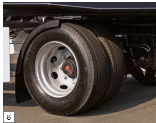
Premium single tyres for 9t axle load, optional: twin tyres for 10t axle load
