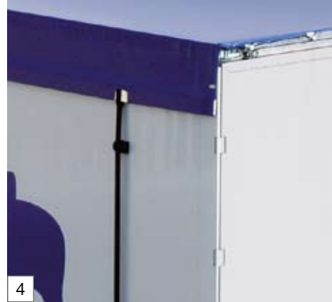
Roller tarpaulin with aluminium winder board
