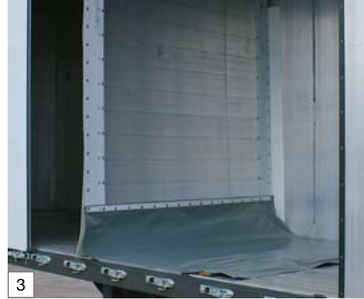
3 Moving wall for complete emptying, option: moving rail cleaner in the upper guide
