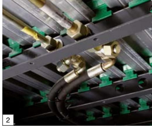
2 Hydraulic fittings on the cross member of the chassis frame at the height of the semitrailer landing gear
