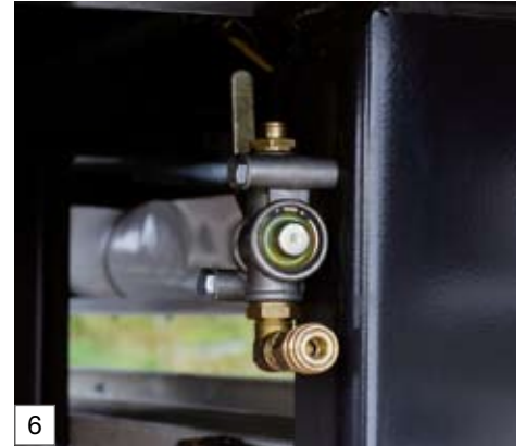
6 Compressed air connection in the rear section with isolating valve
