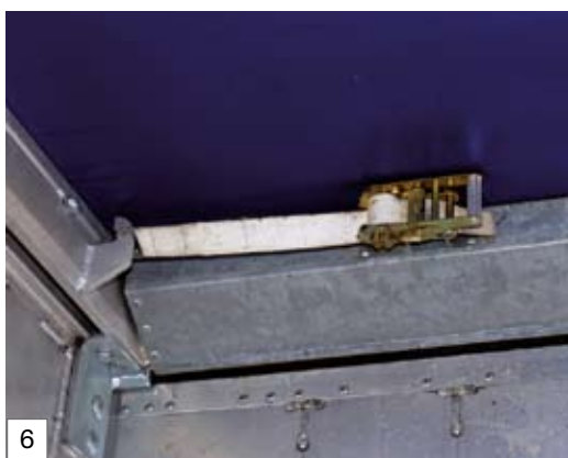
Pivoting upper transverse beam above the rear door with pick-up function provided by tensioning belt and ratchet
