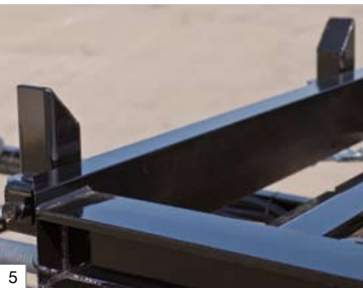
Square plug-in section as front stop for the slide (3 positions)
