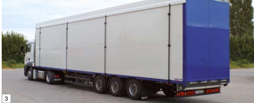
Volume-body with 98.4m 3 cargo volume. Option: Volume-body with 100m 3 load volume, upper strap with delta strip heightened
