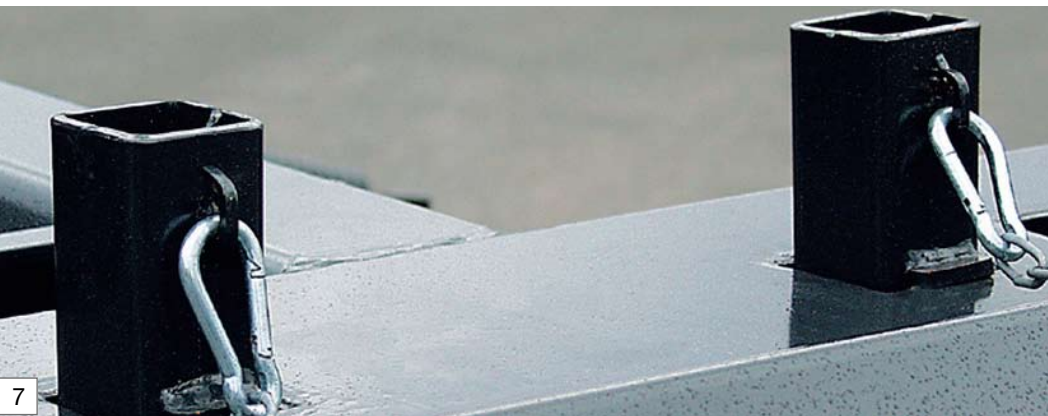
Plug stops – plugged in front of and behind the container roller, provide additional securing for the container
