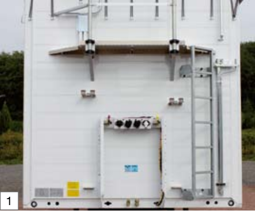
Aluminium bulkhead with working platform, broom and shovel brackets, access ladder right, left or on both sides
