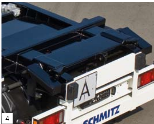
Slide with roller guide and lock
