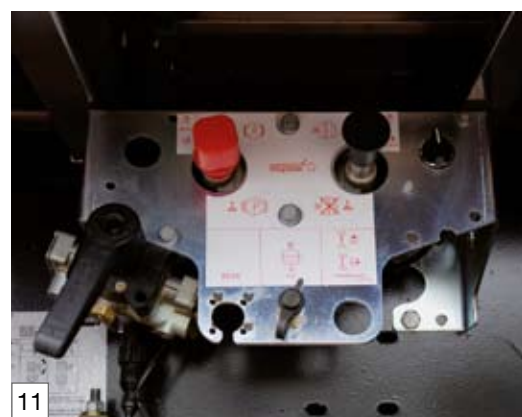
11 Operating console for pneumatic suspension, axle lift and spring-loaded brake
