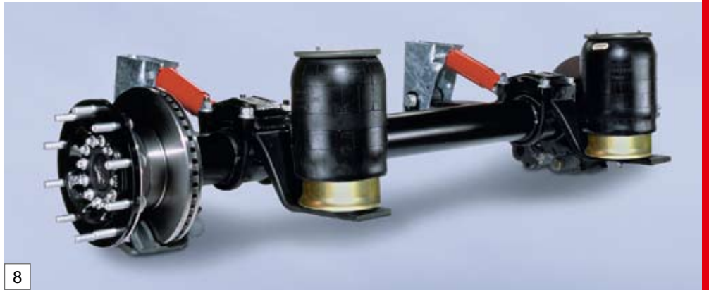
ROTOS® running gear with large 22.5" internally ventilated disc brake, wheel offset 120 mm, running height regulation using Schmitz Cargobull Multi-Ride-Height (MRH) pneumatic suspension, electronic brake system (EBS) and Roll Stability Program (RSP) fitted as standard
