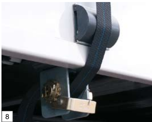
Tarpaulin securing using tensioning belts and ratchets
