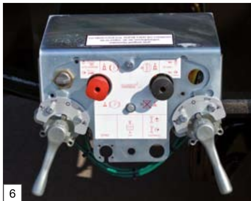
Control unit for parking brake and pneumatic suspension with 2 lifting & lowering valves and container locking
