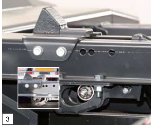
The crank guided 4-point hook lock clamps the container on the chassis
