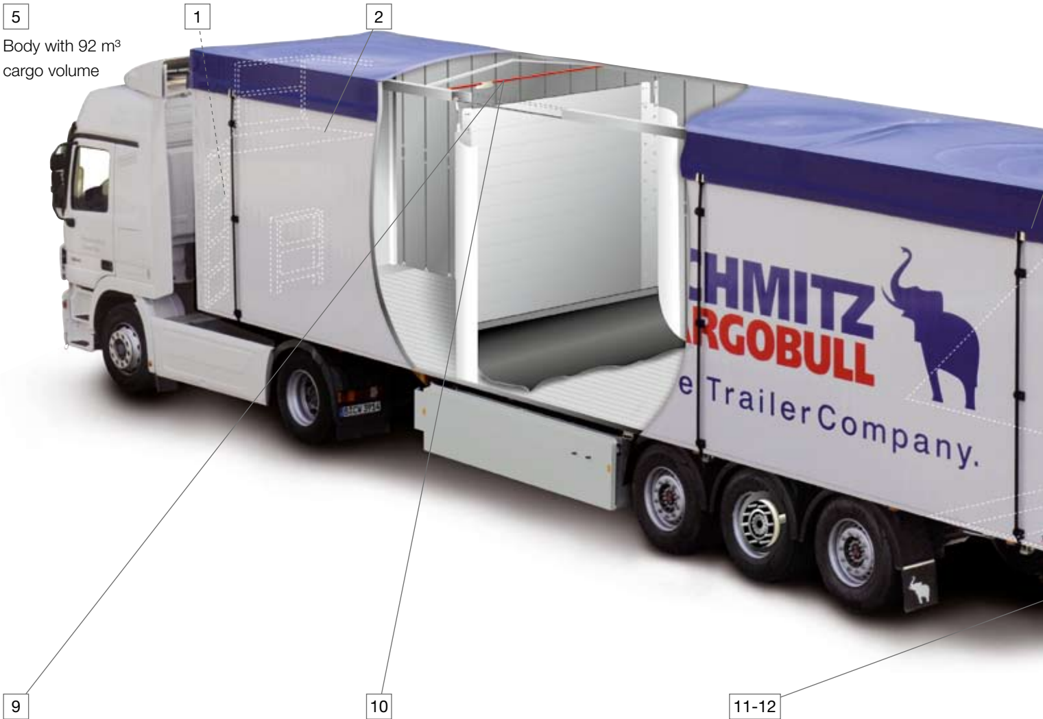
Aluminium bulkhead with working platform, broom and shovel brackets, access ladder right, left or on both sides
